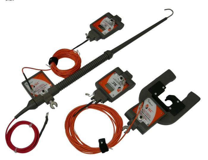
The LiteWire sensors are suitable for MTE's meter test equipment PRS 400.3, CALPORT 300, PWS 3.3, PWS 2.3 PLUS and PTT 2.1. The LiteWire is a true RMS meter designed for use by electricity utilities to sense currents or voltage waveforms from the primary side of their distribution networks. A fiber optic link transmits information as well as establishes isolation between the high voltage potential at the sensor enclosure.
